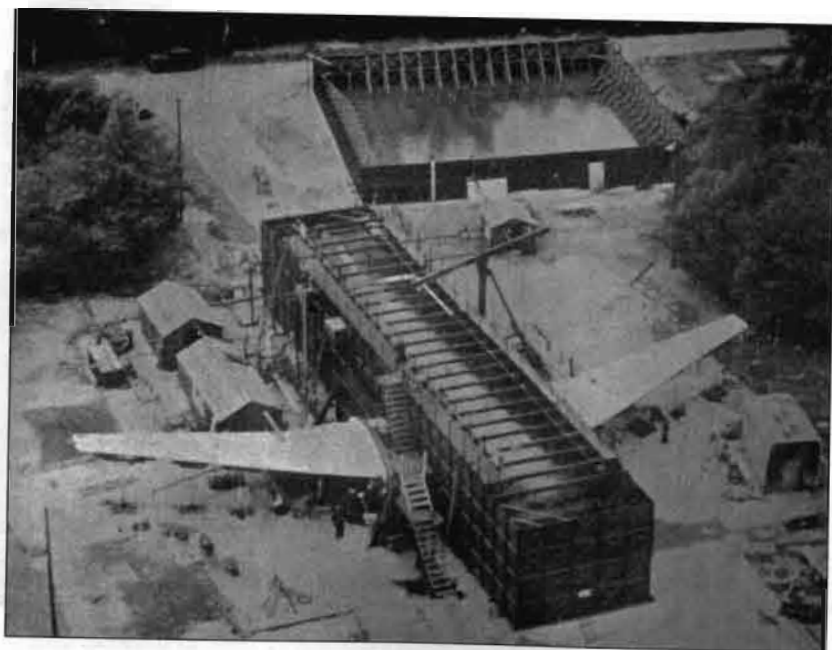
At the Royal Aircraft Establishment in Farnborough, England, workers test a Comet fuselage in a water-filled tank. | (Photo courtesy British Aerospace Hatfield)
