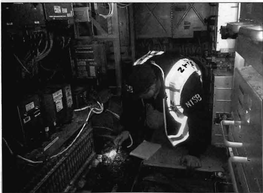
NTSB investigator Mike Bauer examines the damage from the uncontrolled heating of a lithium-ion battery on a JAL 787. | (Dreamliner NTSB photo)
